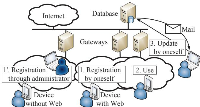
Fig. 2. Usage Flow of the Proposed System
